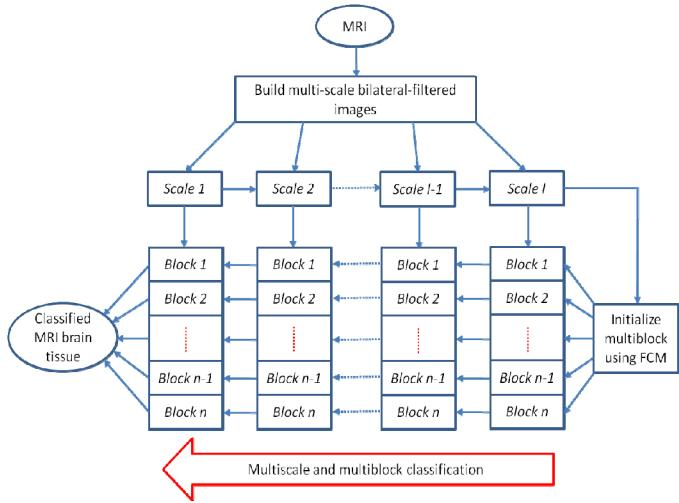
Fig. 1. Schematic flow chart of the proposed MsbFCM method.
