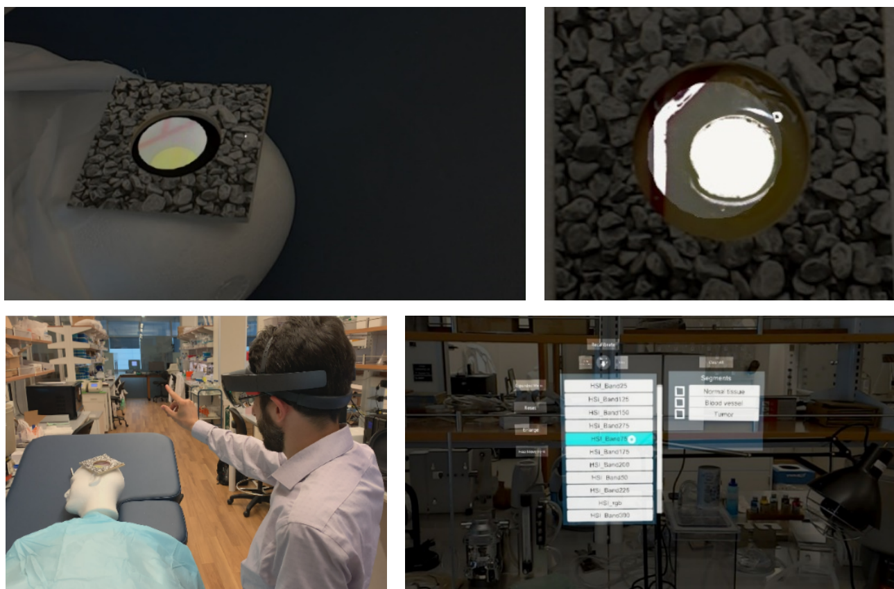
Figure 8. The HoloLens application creates a convenient and untethered method to visualize tissue segmentations in real time. The top two images shows the segmentation labels overlaid on top of the brain tumor phantom. From the images, it can be seen that the boundaries of the blood vessel and tumor are clearly defined and easily distinguishable from the surrounding tissue. The image on the bottom left shows the scene setup and basic interaction with the application through a finger tap movement. On the bottom right is the application interface as seen through the HoloLens. There is a band selection menu which contains each of the spectral bands in the hypercube as well as a smaller segmentation label menu which allows the user to see the tissue segmentations overlaid on the phantom.
