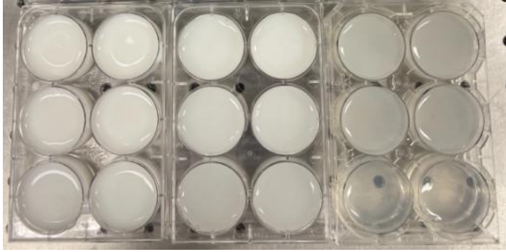
Figure 1. The figure on the left shows the LE phantoms at different concentrations (0% – 10%). The table on the right indicates the specific concentrations for each set of phantoms, with there being two phantoms for each concentration. As the concentration increases, so does the reflectance of the phantoms, thus showing a higher brightness. The 0% phantoms contain no LE, only DI water to obtain a baseline for the scattering properties of the LE.
