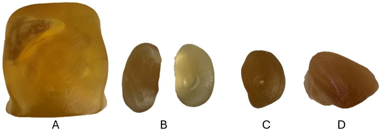
Figure 6. Fabricated phantom models of (A) abdominal surface, (B) kidneys, (C) spleen, (D) liver.
